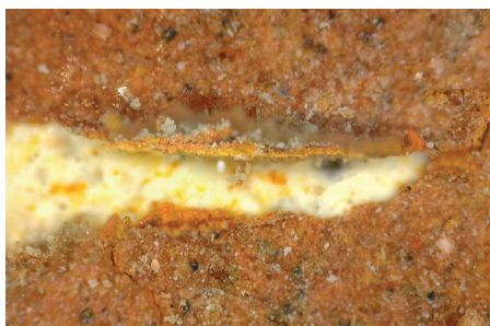
Picture 2. Observation under a portable digital microscope, RAK light. The lifting of the protein intervention material curls the paint film, revealing the white adhesive underneath.
